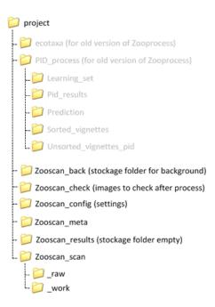
**IMPORTANT**: Create the project on the computer **to which the ZooScan is connected** because when you install ImageJ on a computer connected to a ZooScan, a "ZooScan" folder is created on the C: disk. This folder contains specific information about the connected ZooScan, such as frame dimensions, which Zooprocess needs to integrate into your project.
